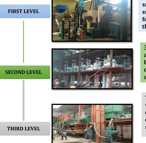
small processing units with a capacity of 0.2 to 2 t/h located in the surrounding of production areas for the production of milled rice for local consumption. There are currently more than 2,000 units throughout the country
