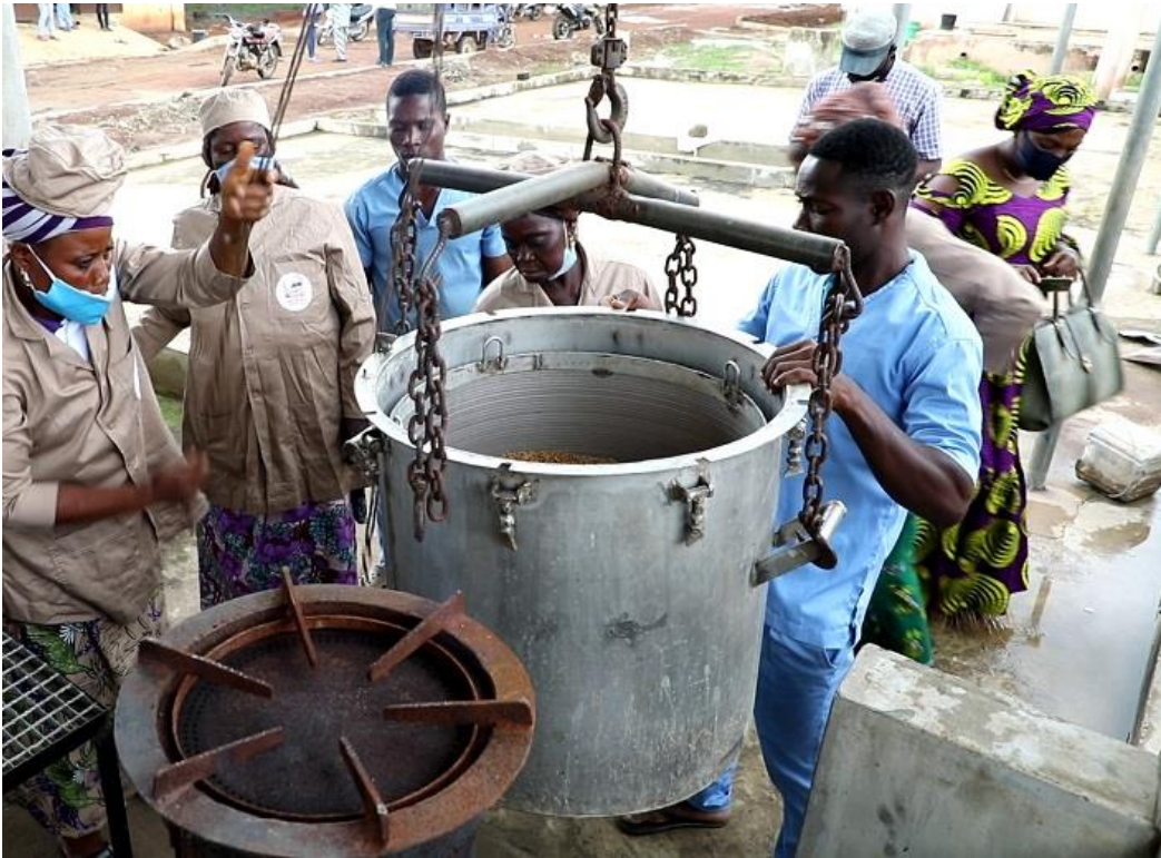
GEM parboiler technology in operation at the Glazoue Innovation Platform in Benin Republic (PHOTO: TAAT/Atayi Opaluwah)
