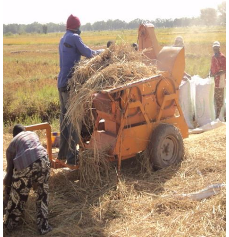
Locally manufactured AS thresher, by CDARMA Dosso, from an imported prototype from Senegal.
