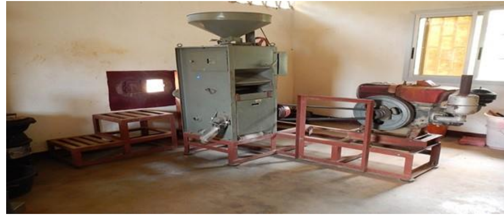
SB10 mini husker installed by a support project in an emerging rice-growing basin
