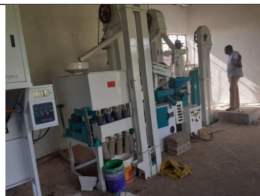
Figure 9: Multi-stage combination rice mill with milling capacity of 1.5MT/hour
