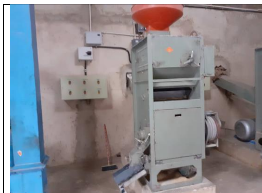
Figure 8: Satake SB 50 milling capacity 1.8 – 2.3 MT/Hour
